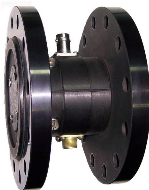
The MA20 torque transducers are used to measure static and dynamic torque in a non-turning mode. They are suitable for use in testing machines as reaction torque transducers or in calibration devices as reference torque transducers.
