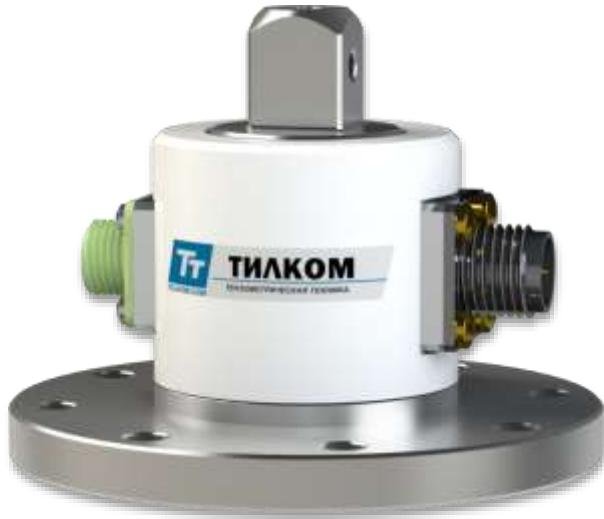
The MA20B is non-rotating torque transducer with the mixed connecting ends. It has a flange end at the one side and a square at the other side. The square end is produced according to ISO 1174-2.
